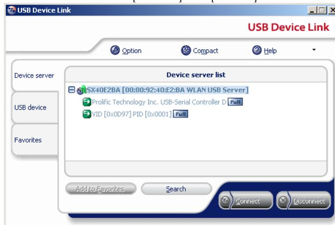
We need to connect to the devices so the computer you are using thinks the USB devices are connected directly to it. Click on the USB2Serial adapter entry and click the “Connect” button.
