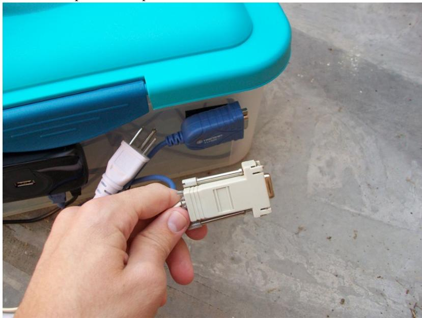
Below shows the telescope's cable connected to the adapter. The other side of the USB2Serial adapter should already be connected to the black USB hub.
