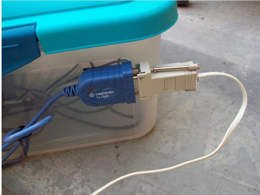
Connect the serial cable from the SBIG CCD Camera to the black USB hub. Below shows the camera's cable connected to the USB hub.
