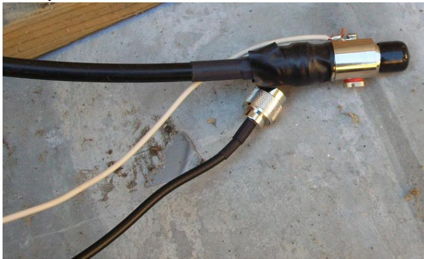
Below is a picture of the antenna connectors connected with the plastic cap on the ground below.
