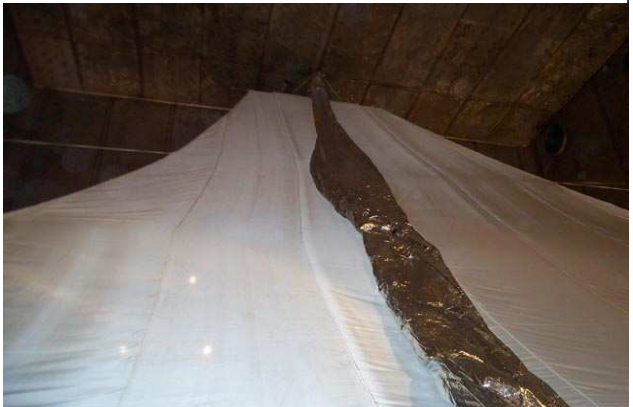
Solar sail deployed in the vacuum test chamber at NPO Lovochkin. Credit: © Louis Friedman and the Planetary Society
